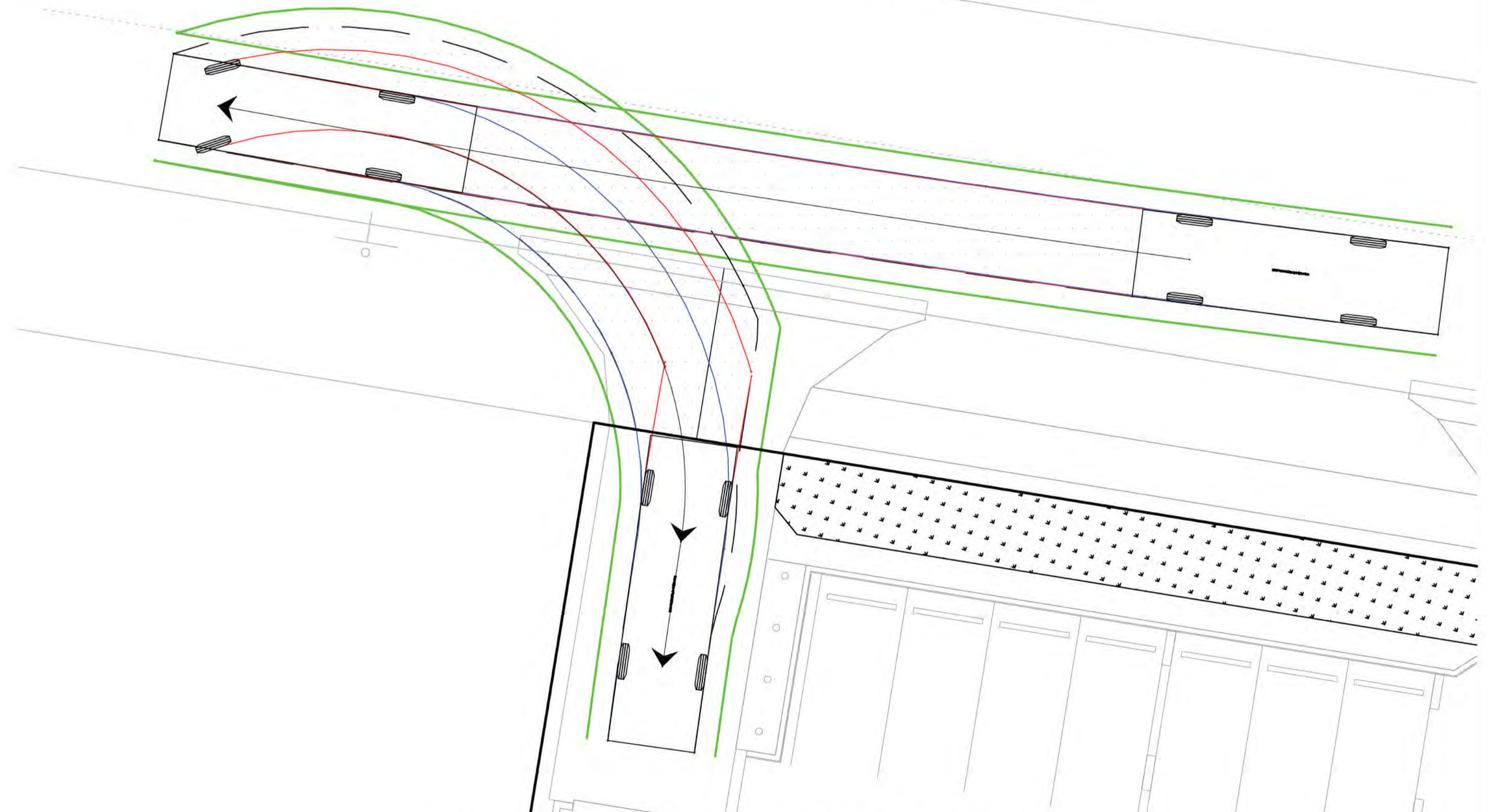
MEDIUM RIGID VEHICLE - 8.8m SERVICE VEHICLE - REVERSE IN SCALE 1:100
