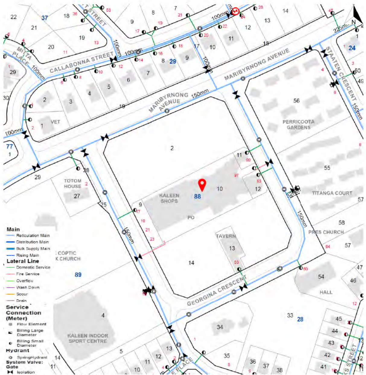
Figure 17 – Existing Water Infrastructure Near the Subject Site (Icon Water, 2024)
