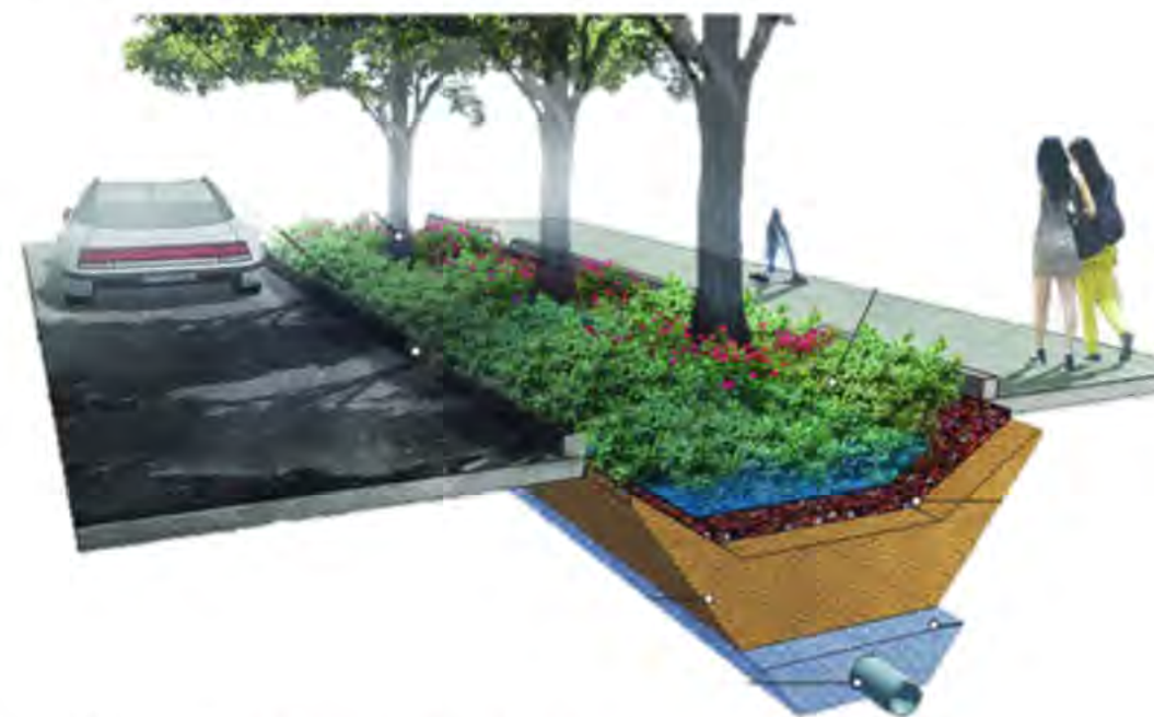
Figure 8.4 Typical Raingarden Cross Section
