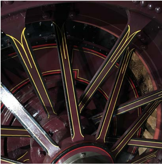
Image 9 Pin striping and new paint on wheel (ACT Heritage 2016).
