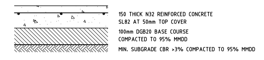
150mm CONCRETE PAVEMENT NOT TO SCALE
