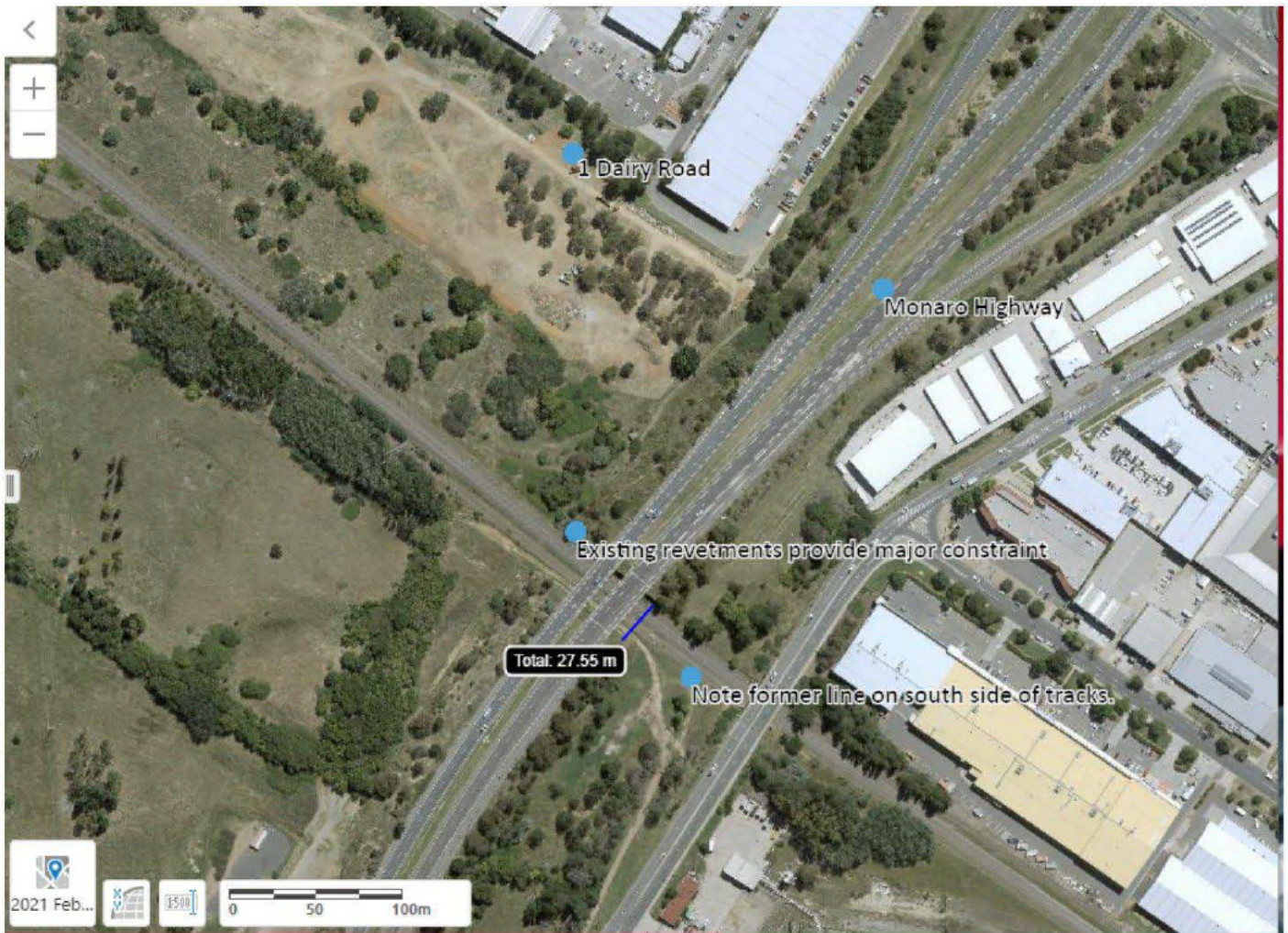
Aerial photo showing constraints imposed by existing rivetments of Monaro Highway overpass. Source ACTMapL.
