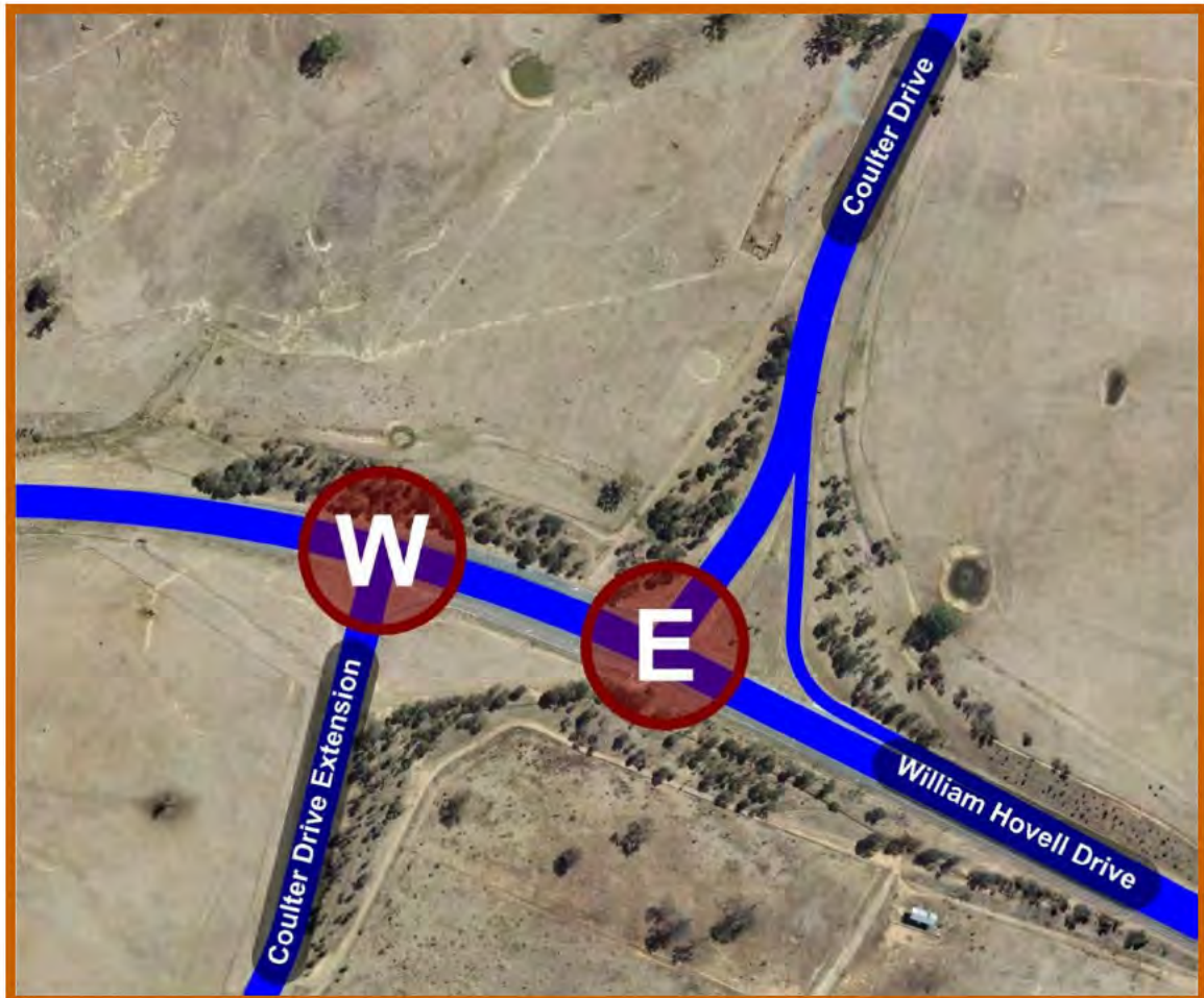
Figure 104: Staggered T Intersection Layout
