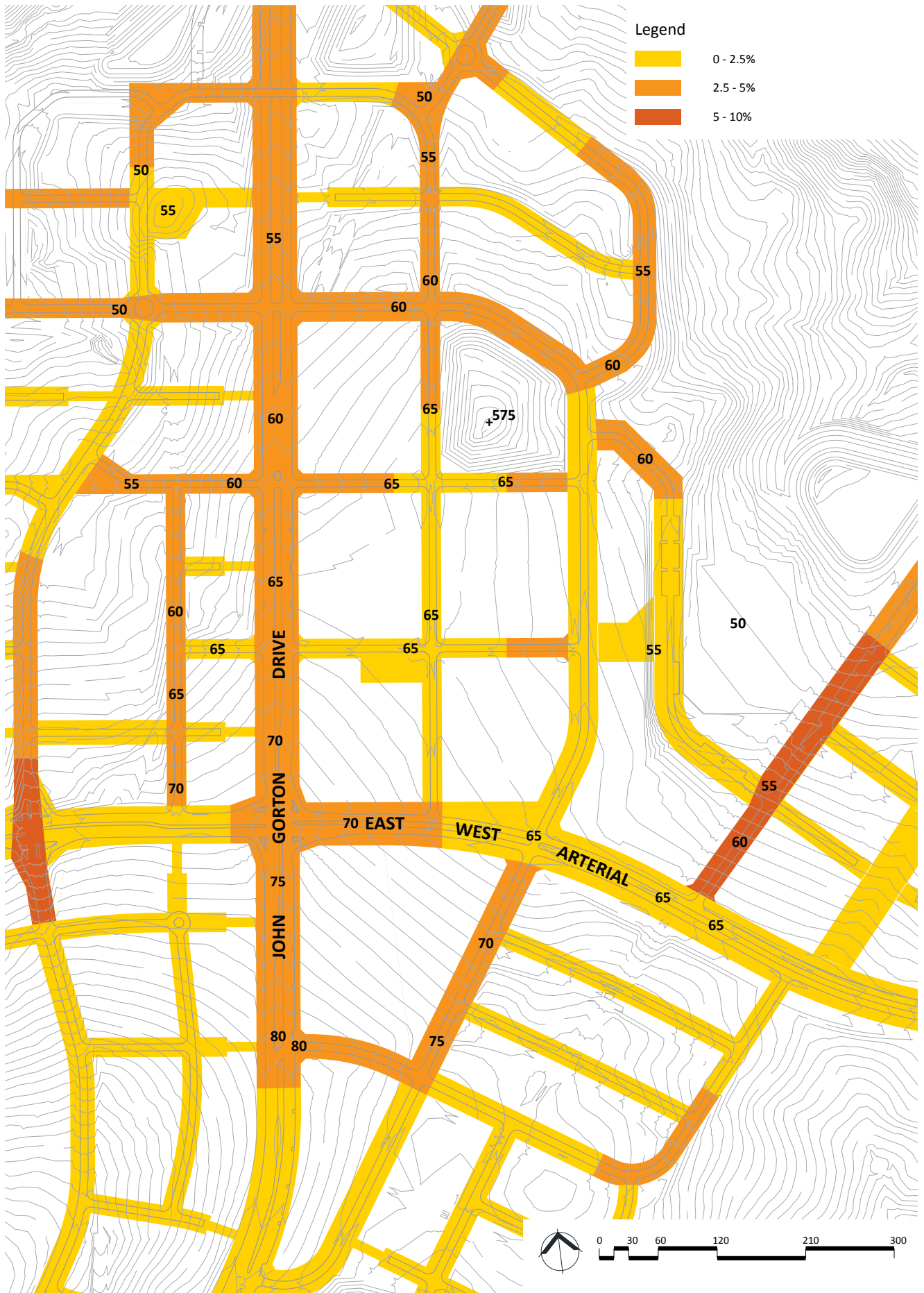
Figure 19: Grading and universal access
