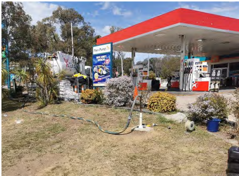
Figure 8 MPVE trial setup showing the stinger entering the extraction well head.
