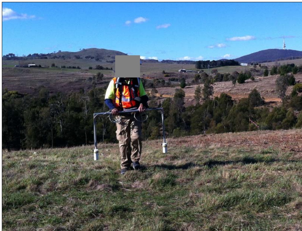
Figure 8: Data Collection Using G858 with integrated DGPS
