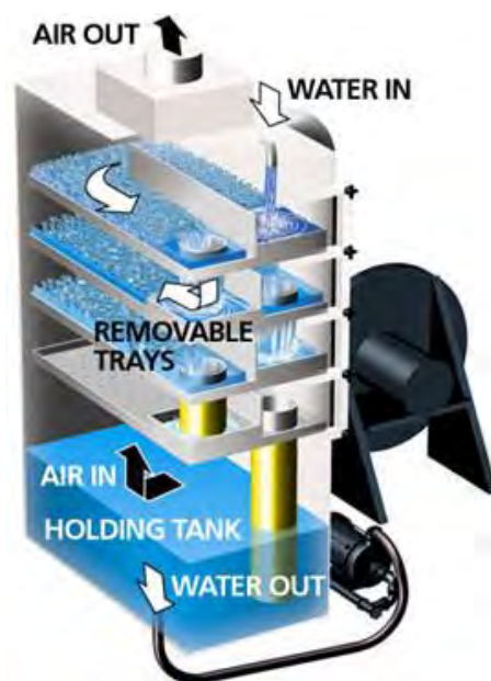
Figure 4 Example of an air stripping unit.
