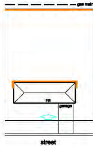
10. MAIN AT REAR OF BLOCK
