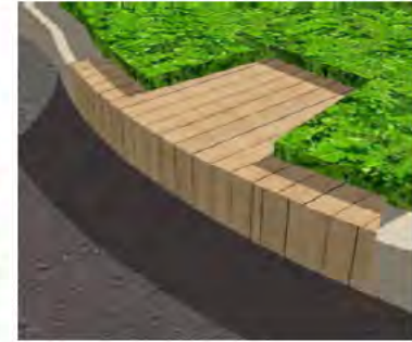
Timber decking rest platform
