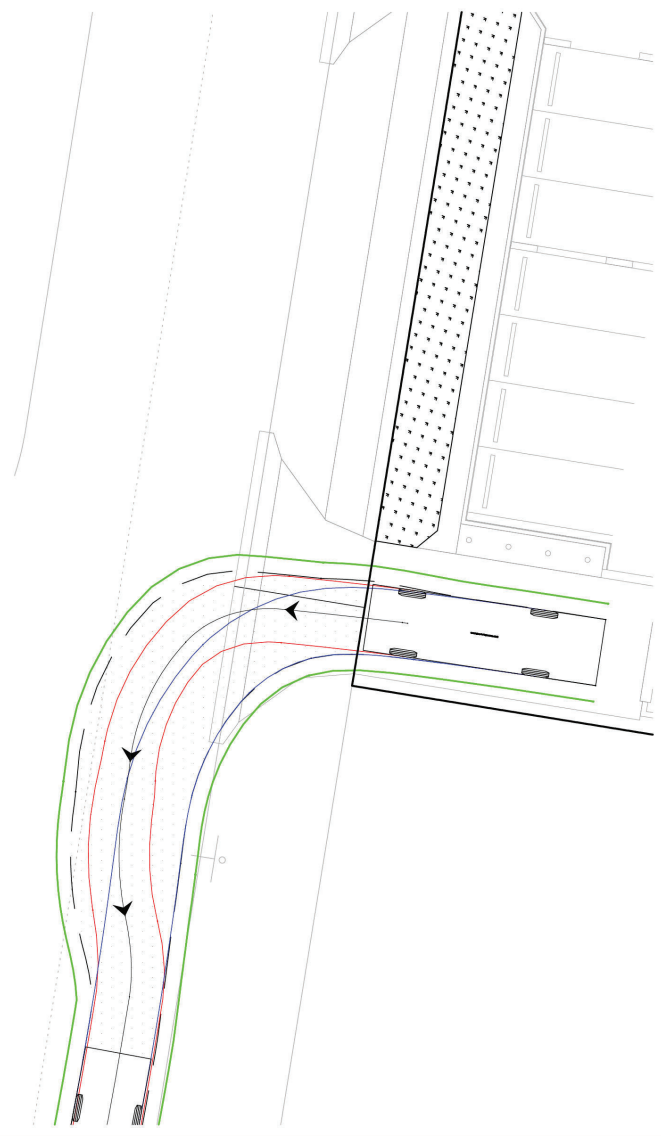
MEDIUM RIGID VEHICLE - 8.8m SERVICE VEHICLE - FORWARD OUT SCALE 1:100
