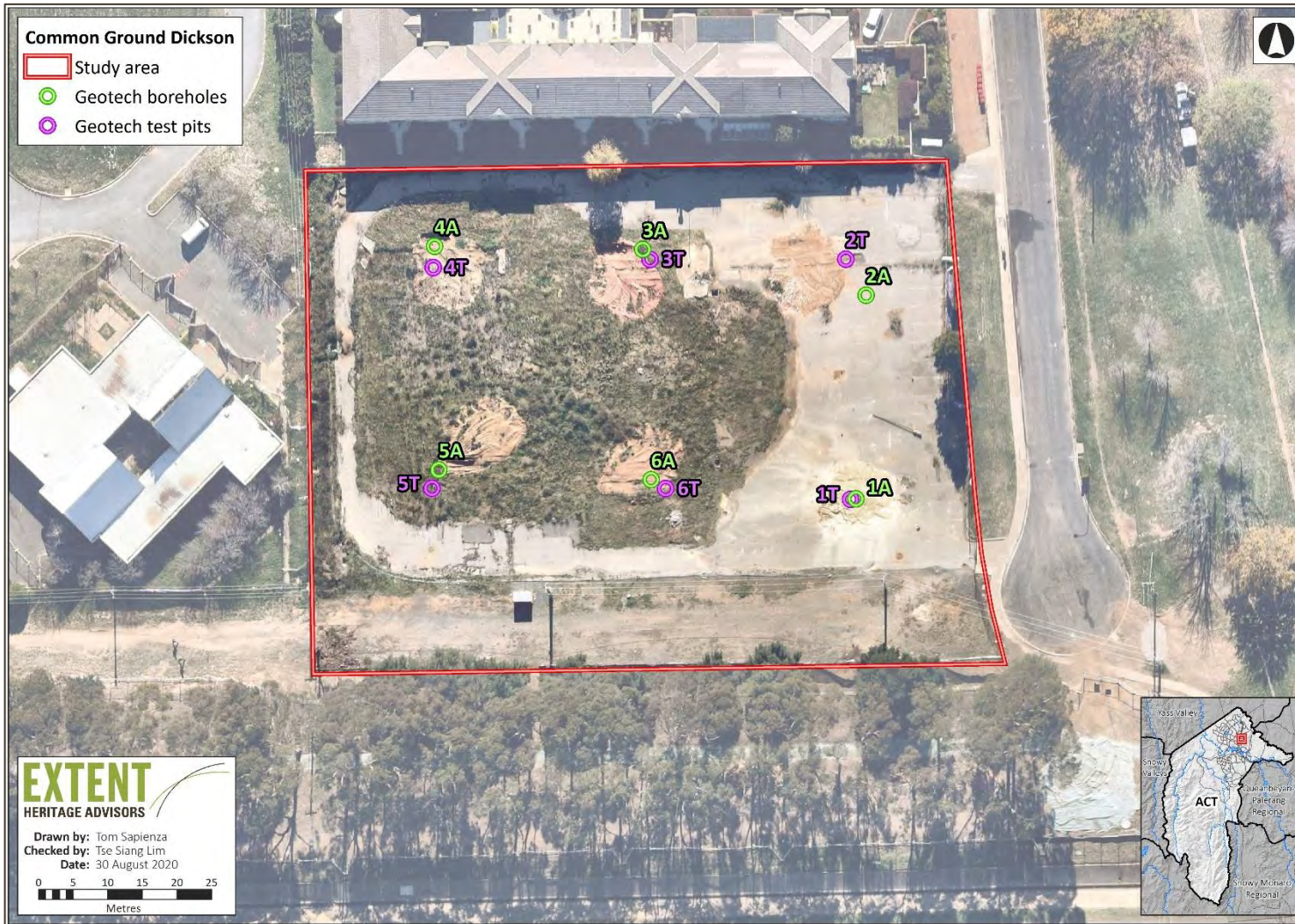
Figure 7. The location of the six boreholes (1A-6A; ACT Geotechnical 2019a) and six test pits (1T-6T; ACT Geotechnical 2019b) across the study area (outlined in red).
