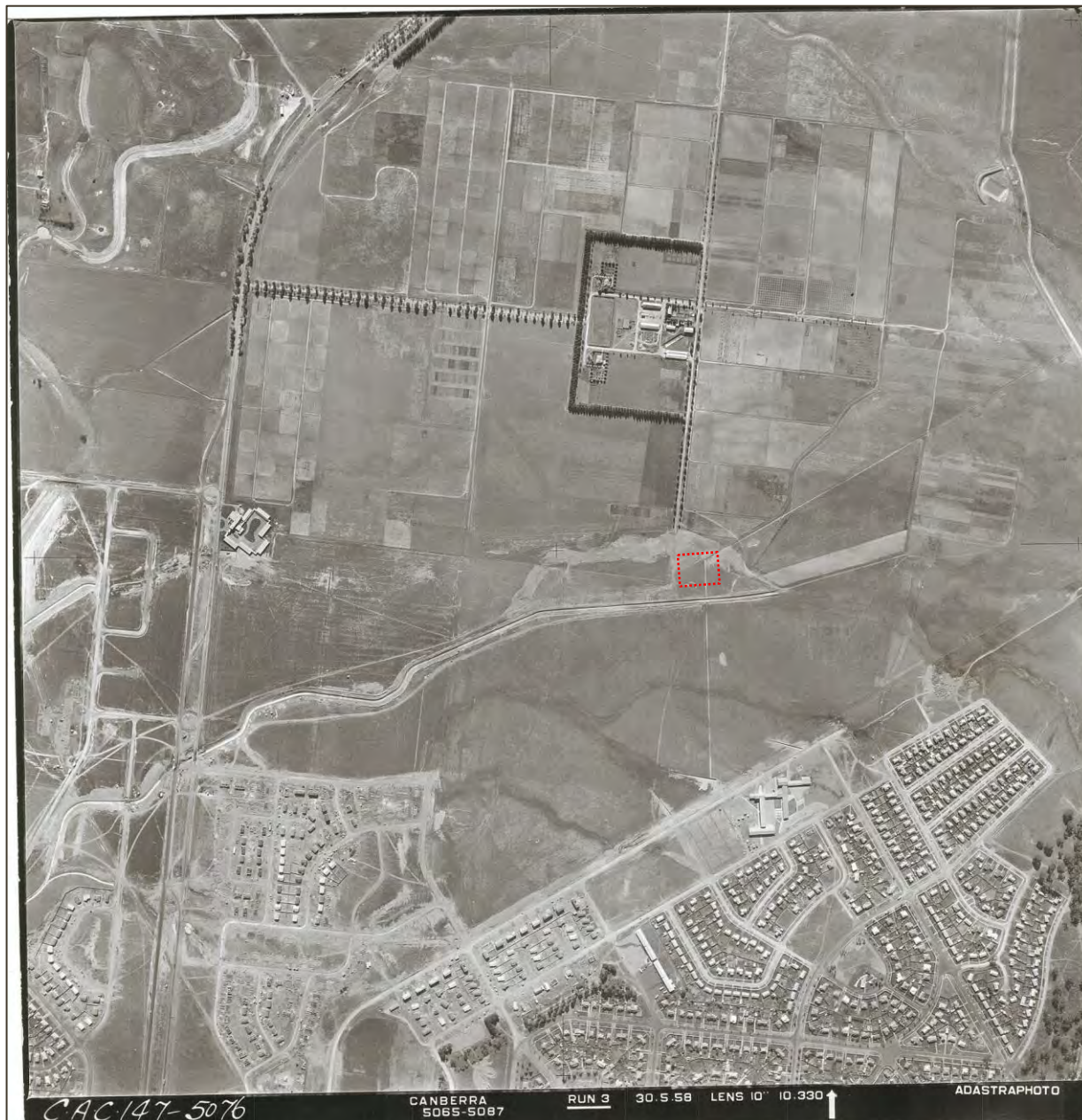
Figure 14. Aerial imagery of the study area (outlined in red) and encroaching urban development to it south in 1958. Note the relocation of the creek line from the north boundary of the study area to its south as part of its conversion into the present 'Dickson Channel' stormwater drain in conjunction with the establishment of the Dickson residential suburb (Source: ACTmapi).
