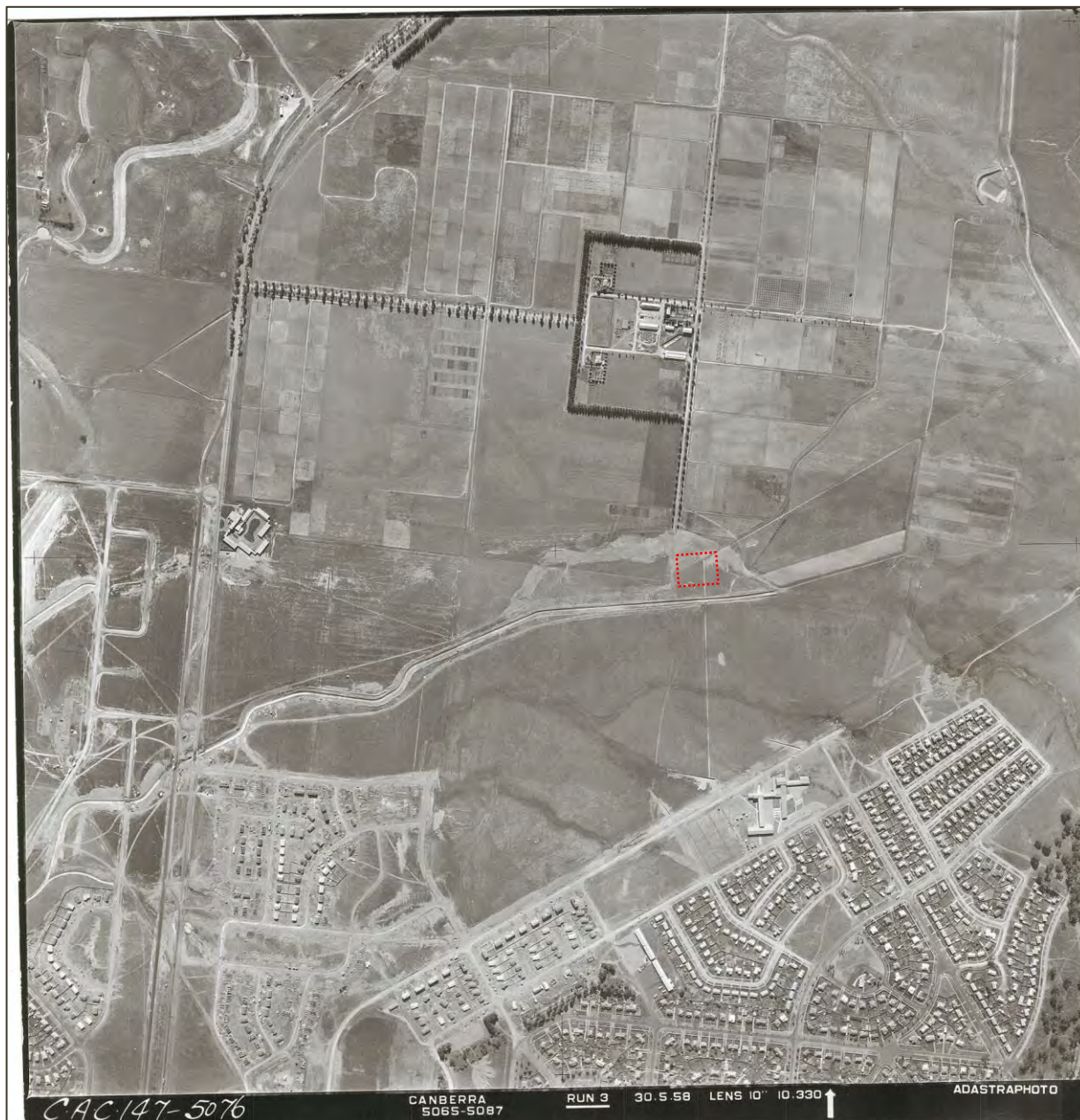
Figure 9. Aerial imagery of the study area (outlined in red) depicting rapid urban development around it in 1958. Note the relocation of the creek line from the north boundary of the study area to its south as part of its conversion into the present 'Dickson Channel' stormwater drain in conjunction with the establishment of the Dickson residential suburb (Source: ACTmapi).
