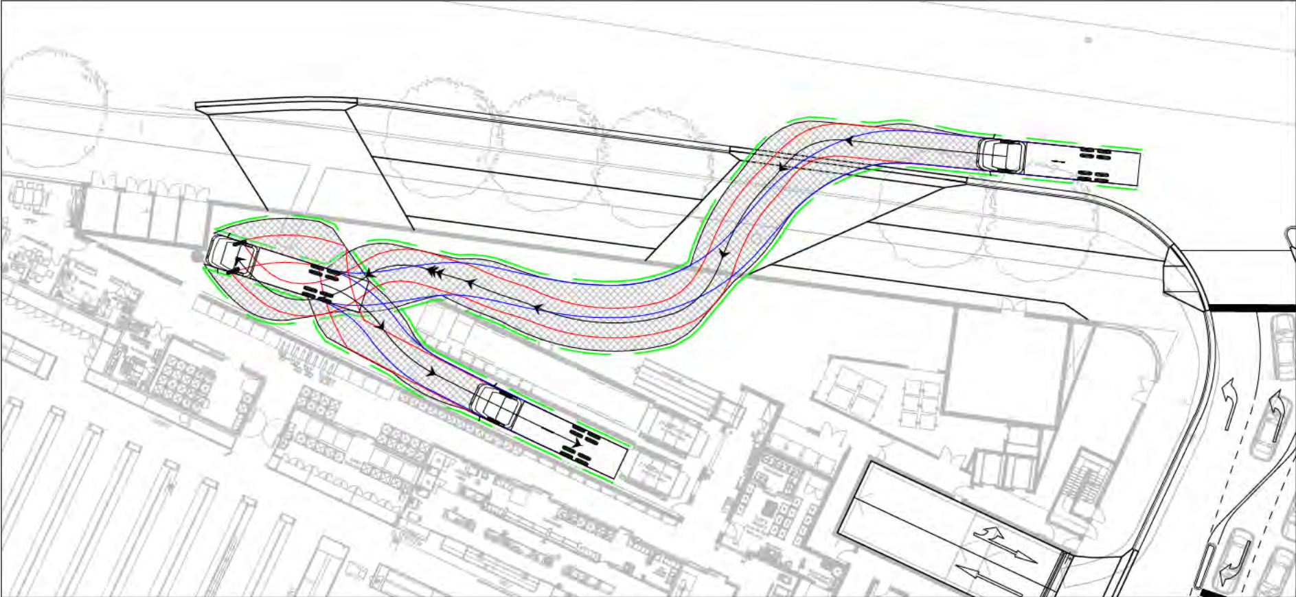
12.5m HRV ENTERING LOADING BAY
