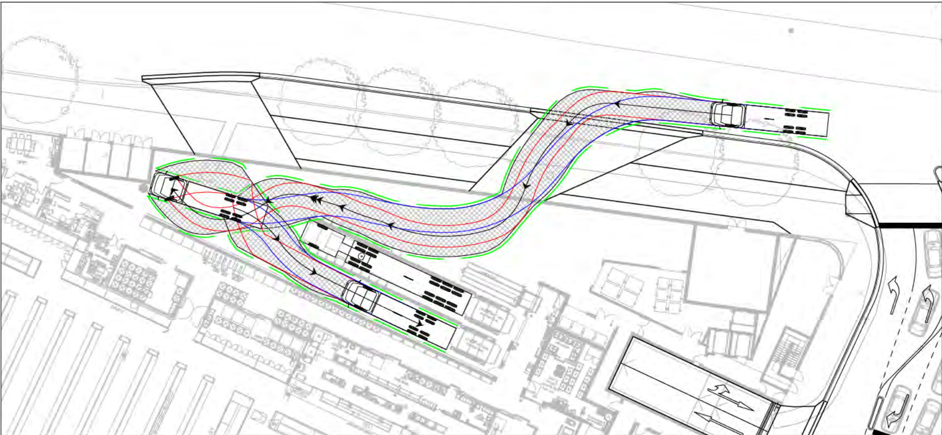
12.5m HRV PARKING ADJACENT 19m ARTICULATED VEHICLE
