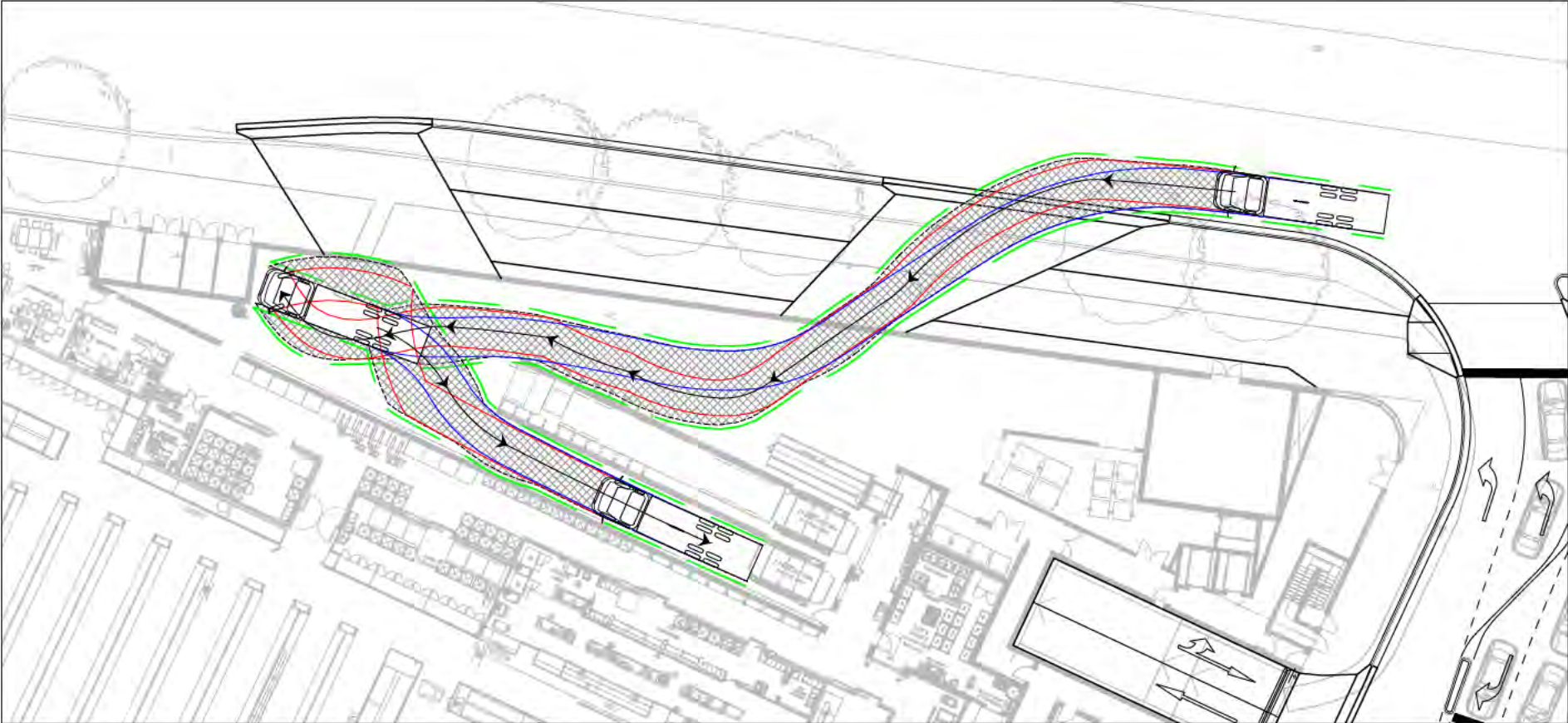
11m HRV ENTERING LOADING BAY
