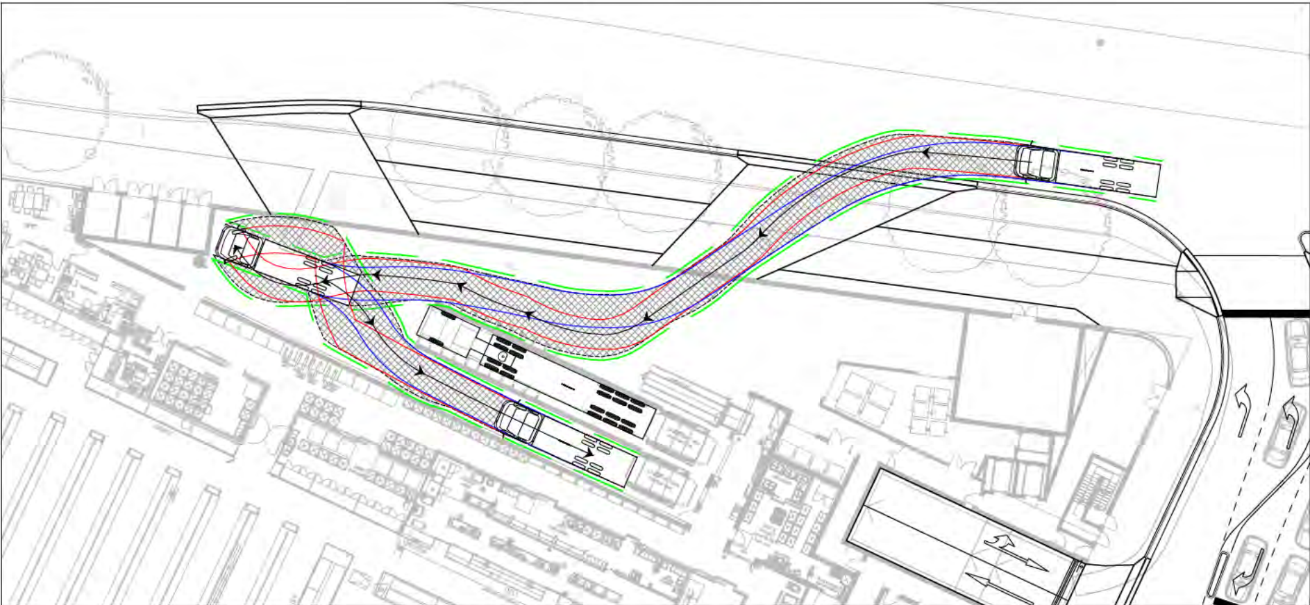
11m HRV PARKING ADJACENT 19m ARTICULATED VEHICLE
