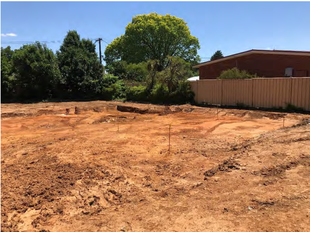
Figure 4 Soil validation sample location/s (from the left) view from the northern elevation of the housing footprint to the western boundary/demolition corner: S05, S06, S12, S07, S11, S07, S08, S10 and S09.
