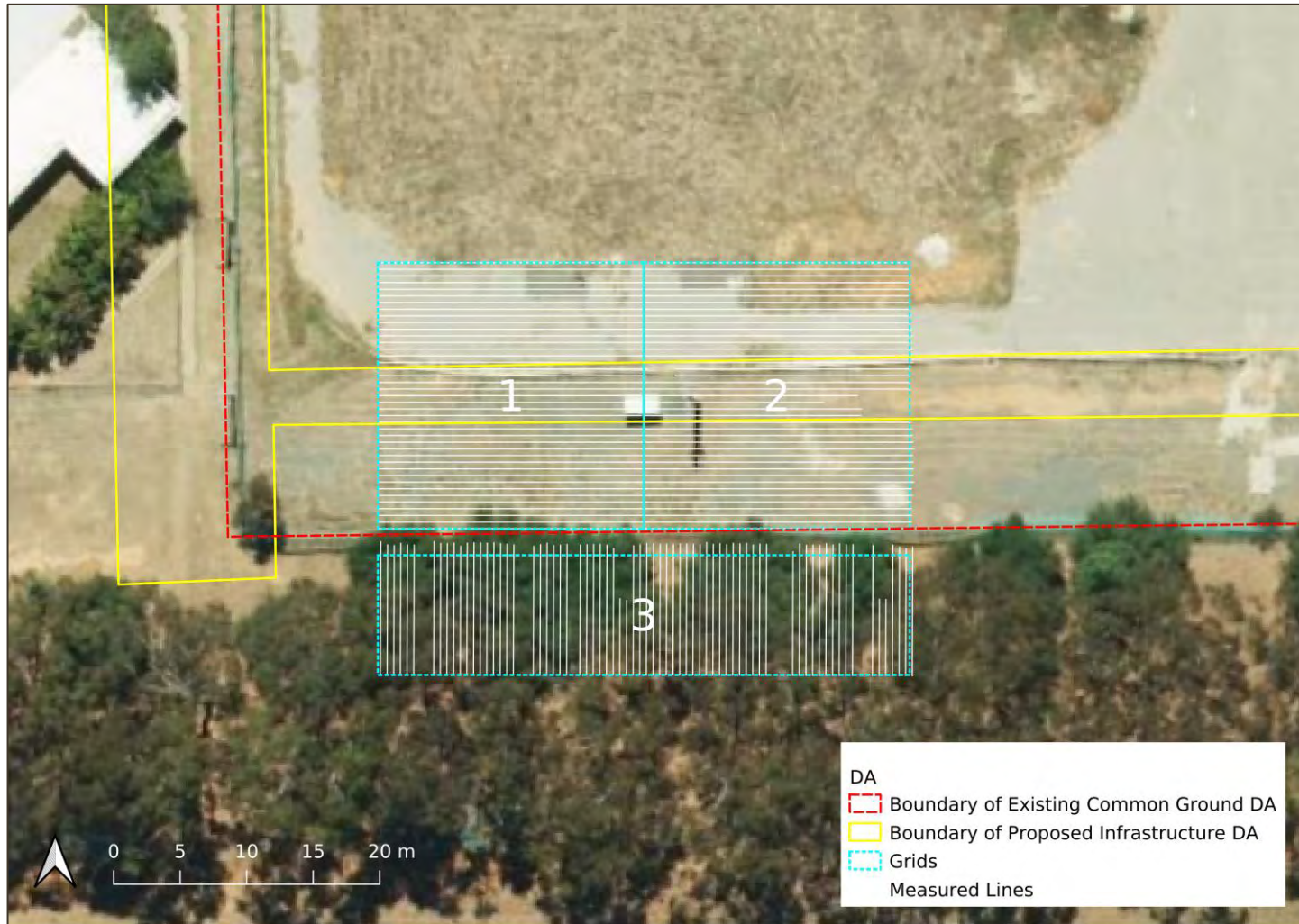
Figure 44. The location of the three ground-penetrating radar (GPR) survey grids (1-3; outlined in cyan) established near the southwest corner of the study area along its south boundary, and the individual GPR survey transects across each of these three grids conducted on 13 August 2020 (outlined in grey) (Source: Geoprospection 2020).
