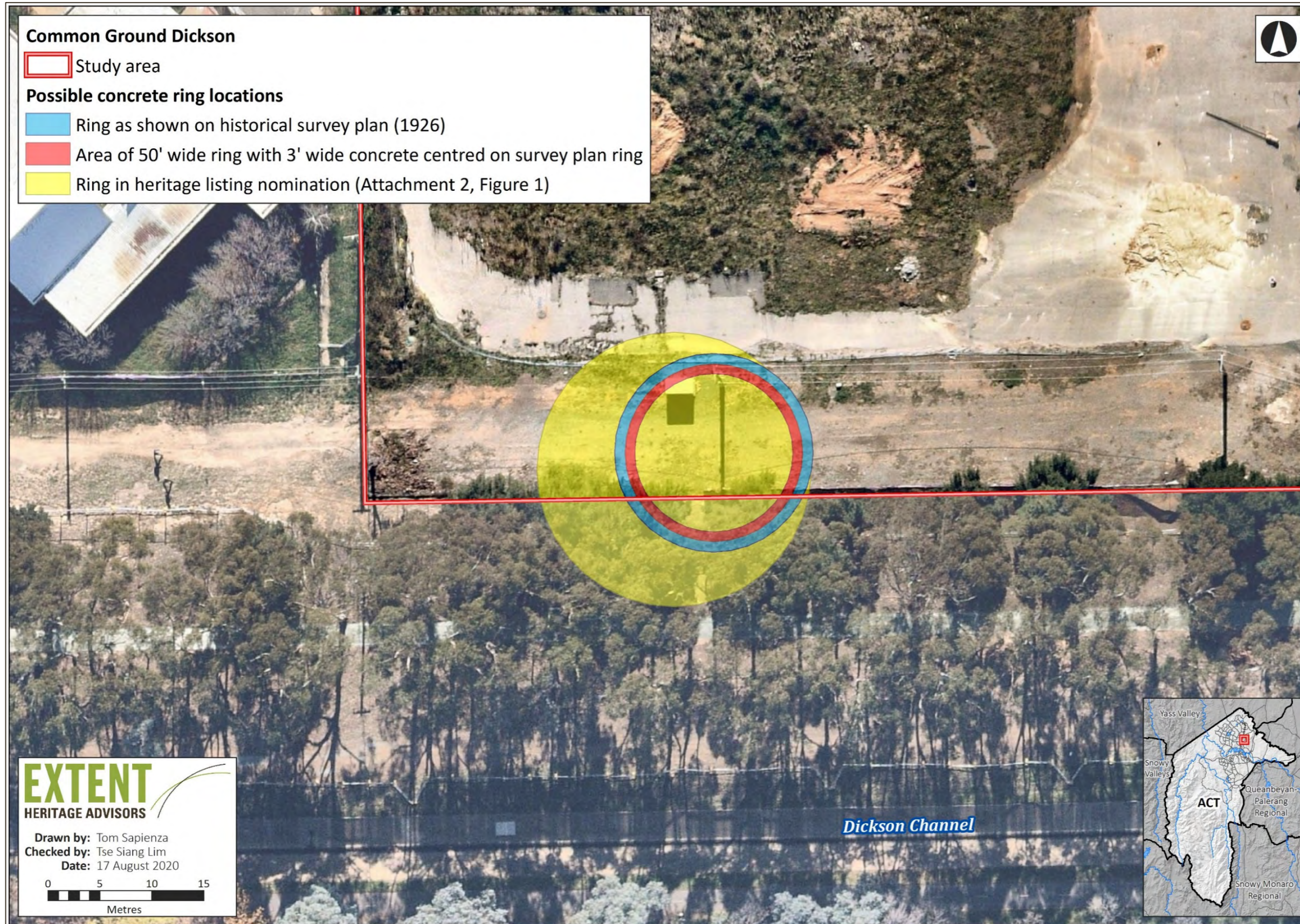
Figure 3. The location and extent of the concrete, whitewashed, central ring marker as indicated on its nomination application for heritage listing (in yellow), as estimated from the 1926 Plan of Contour Survey of Aerodrome Site Canberra (in blue) and its theoretical standard dimensions – a 3 feet wide concrete ring (in red) encircling an area measuring 50 feet in diameter from its centroid – as described in Attachment 5 of its nomination application for heritage listing in the ACT.
