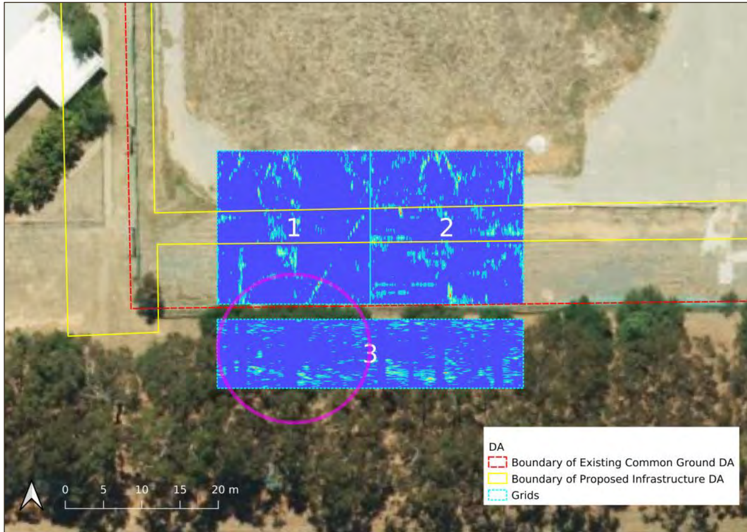
Figure 47. The georeferenced depth-slices at 650 mm beneath ground surface over the three ground-penetrating radar (GPR) survey grids (1-3; outlined in cyan), with an extrapolation of a complete ring from the interpreted presence of Fragments A and B (see Figure 46) indicated in pink (Source: Geoprospection 2020).
