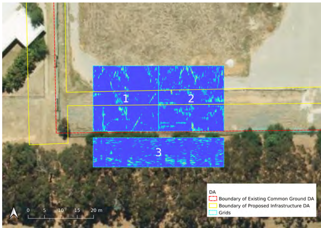
Figure 2: Georeferenced Depthslices at 650 mm showing an arc in Areas 1 and 3. Basemap source: SixMaps.
