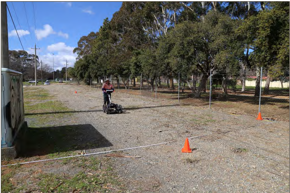
Figure 42. Dr. Sam Player (Geoprospection) conducting the ground-penetrating radar (GPR) survey within and around the historical location of the ring marker at the study area (top and bottom).
