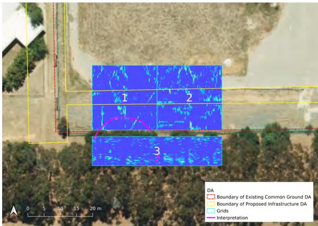
Figure 3: Interpretation of an arc traced over depthslices at 650 mm. Basemap source: SixMaps.
