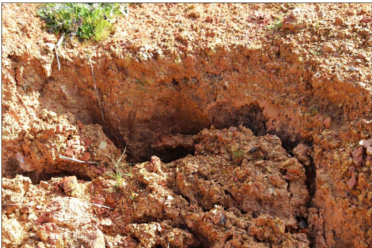
Figure 31. The west view (top) of one of six geotechnical borehole (6A) and test pit (6T) locations, revealing a profile (bottom) comprising reddish clay fill material (c.0-25 cm) overlying dark brown silty sand of the Quaternary alluvium (> c.25 cm) underlying the study area.
