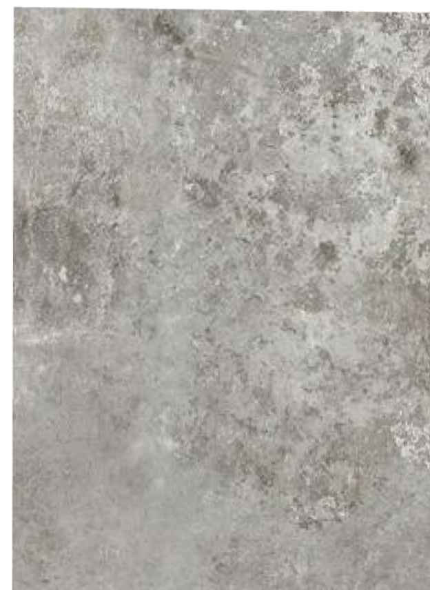
CON 1 CONCRETE OFF FORM NATURAL FINISH
