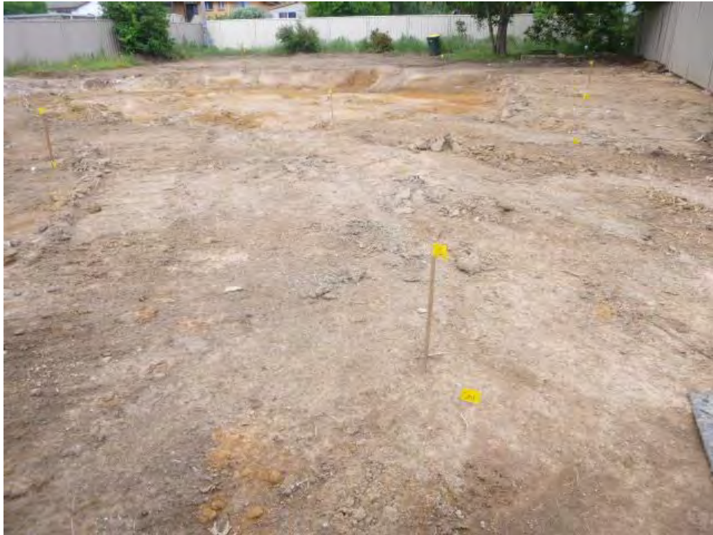
Figure 3 Soil validation sample location/s (from the left) view from the south-eastern boundary to the northern boundary: S02, S10, S12, S09, S08, S04, S07, S01, S06, S05 and S03.
