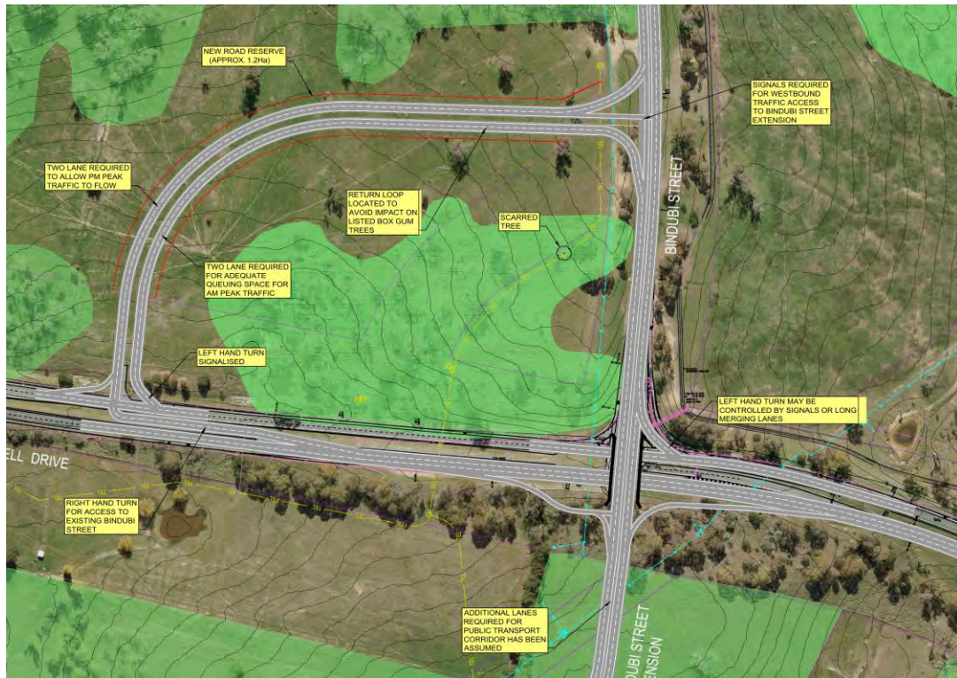
Figure 3: At-grade quadrant intersection with flyover
