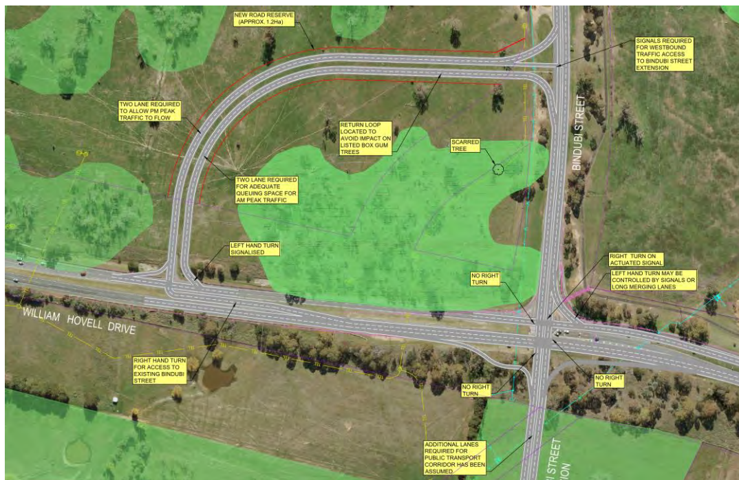
Figure 2: At-grade quadrant intersection
