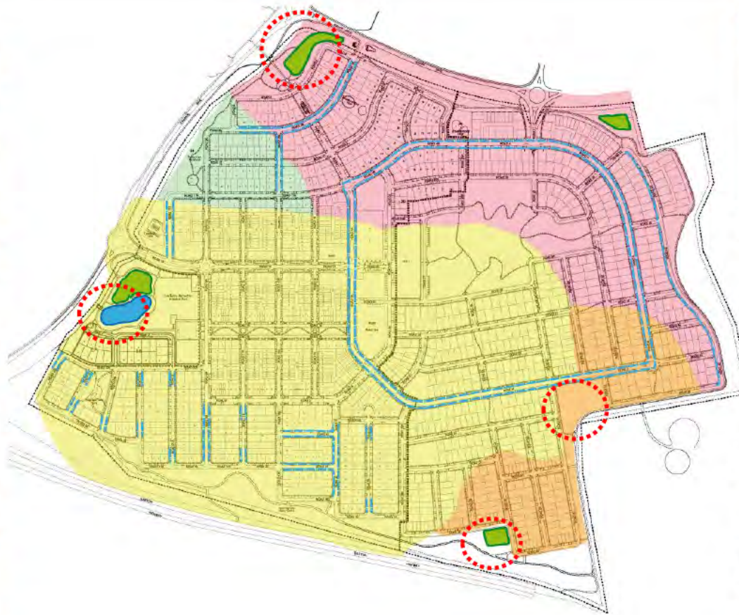
Plan View: Detention areas for Crace in the Northern, Southern and Barton Catchments
