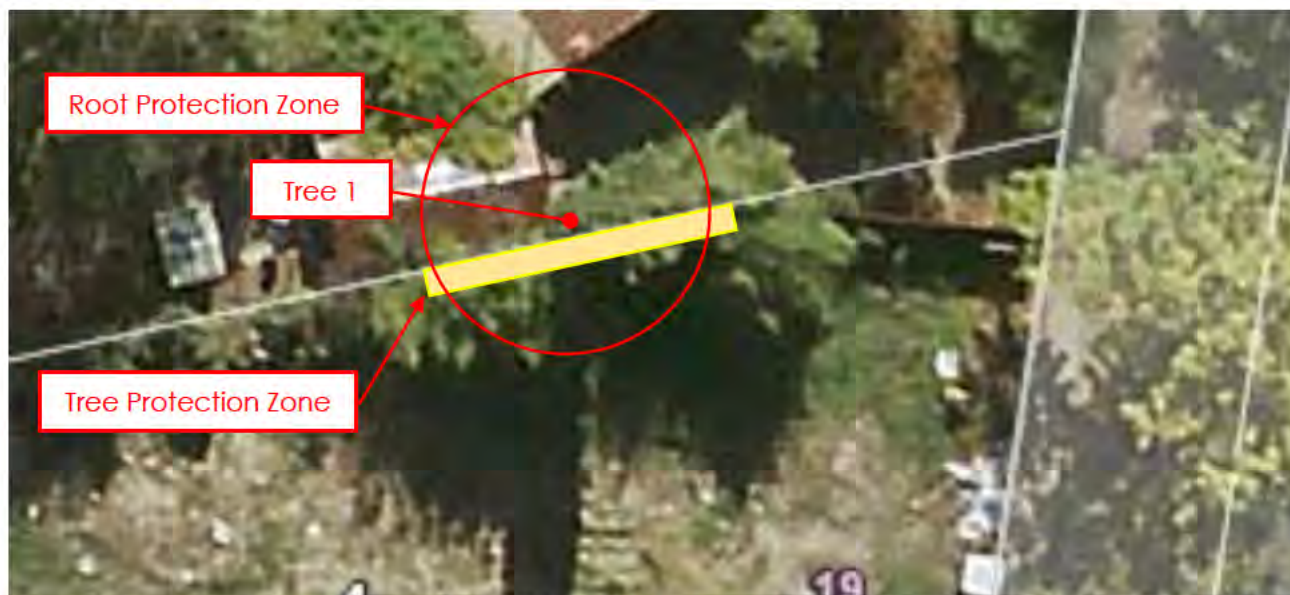
Figure 5. Tree Protection Plan (Drawing) Showing part of Blocks 3 & 4 Section 46, Turner indicating the Tree Protection Zone (TPZ) and Root Protection Zone (RPZ) (not to scale). The RPZ is a circle of radius 5.0m centred on the centre of the trunk. The TPZ is a rectangle 10m x 1m centred adjacent to the tree trunk. The TPZ is to be protected as per TPM 5 - 8 or 10 - 12. Roots in the RPZ are to be cared for as per TPM 16 - 20
