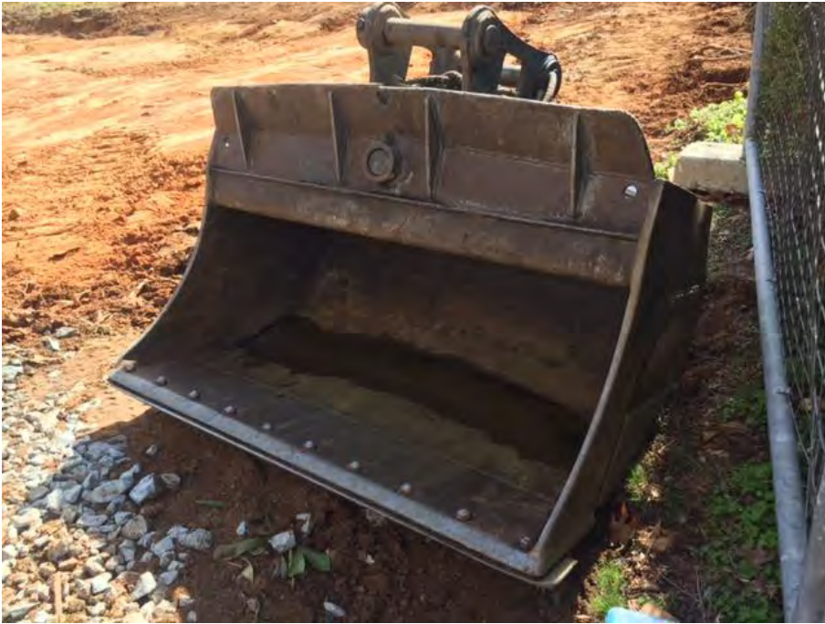
Photograph 5 – Excavator mud bucket attachment after decontamination
