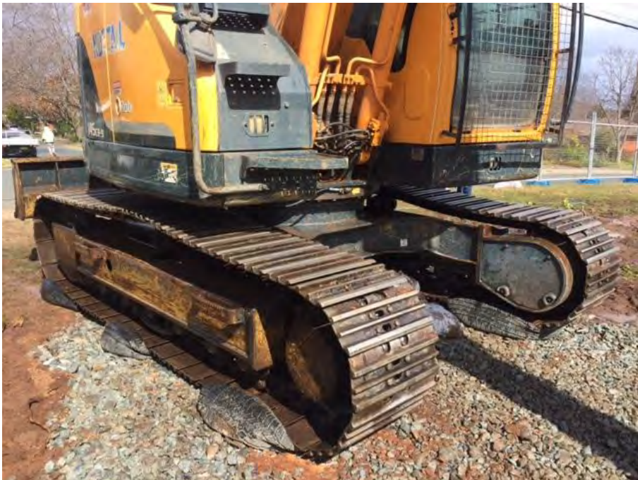
Photograph 8 – Excavator tracks after decontamination
