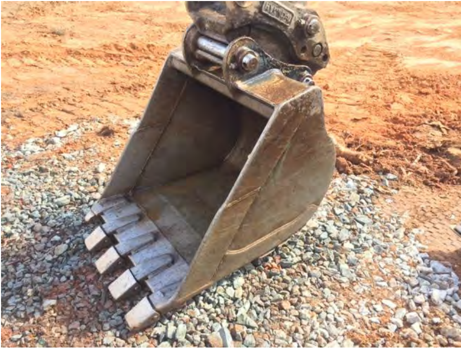
Photograph 7 – Excavator digging bucket attachment after decontamination
