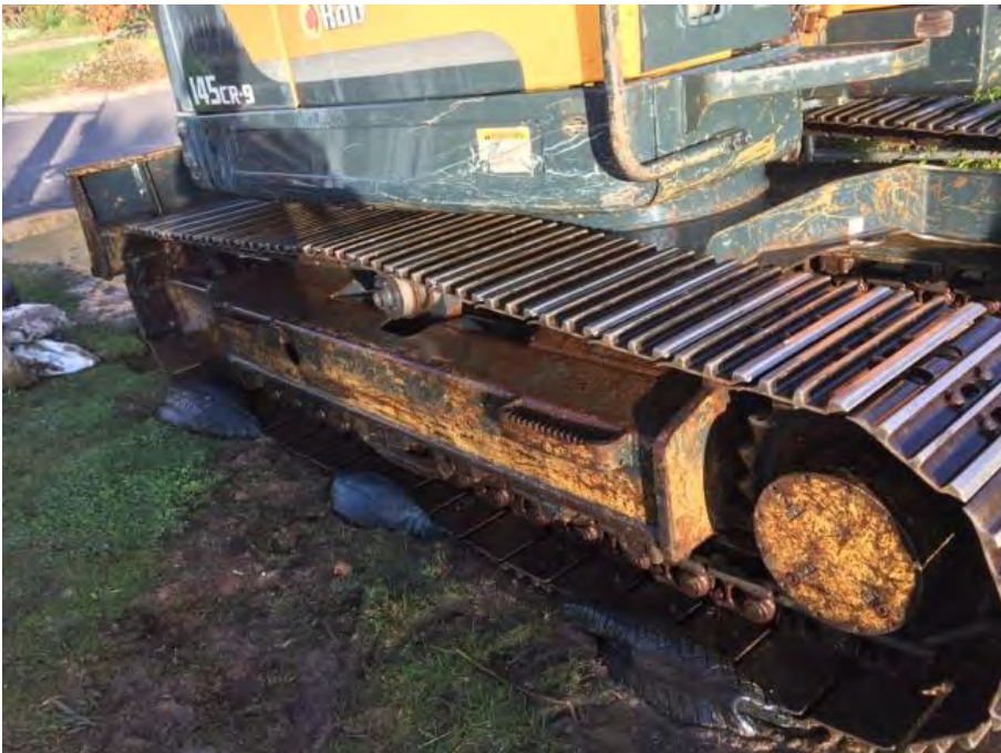
Photograph 8 – Excavator tracks after decontamination
