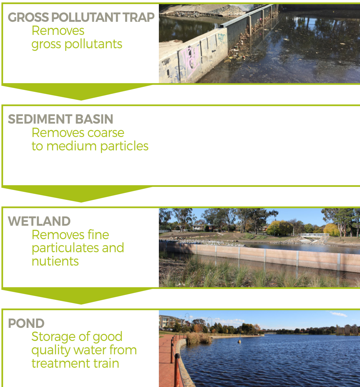
Figure 8: Typical stormwater treatment train adopted in Canberra
