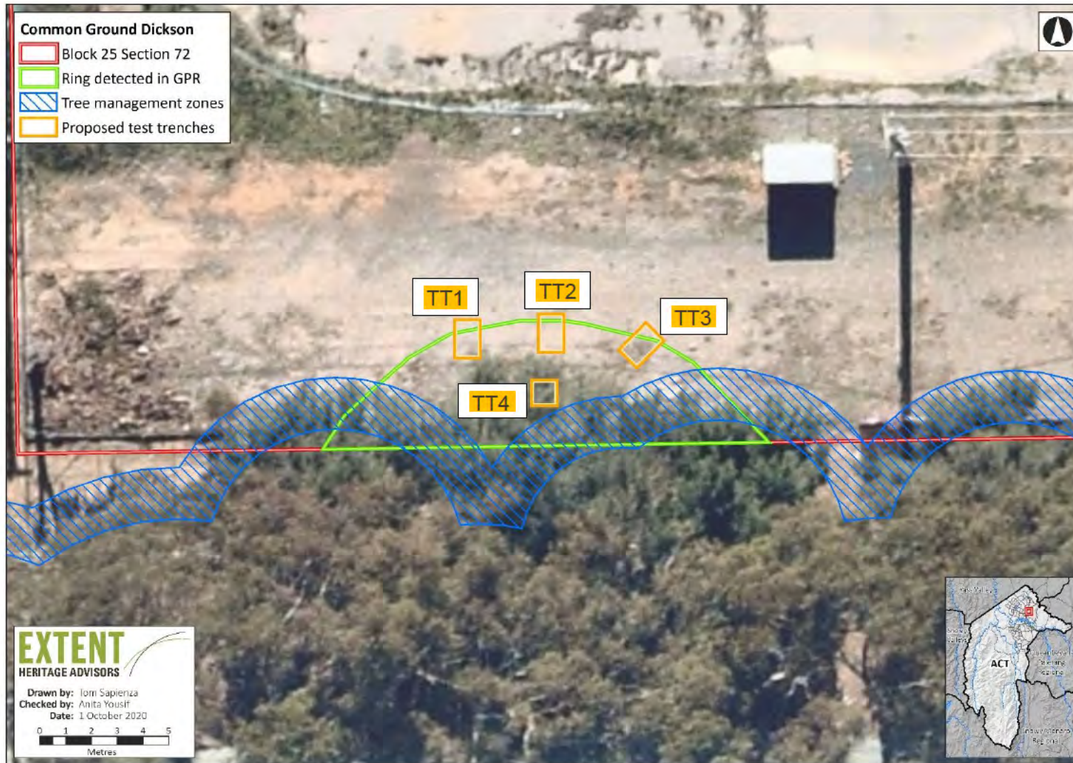
Appendix B. An aerial showing the location of the proposed test trenches relative to the tree protection zone (TPZ)
