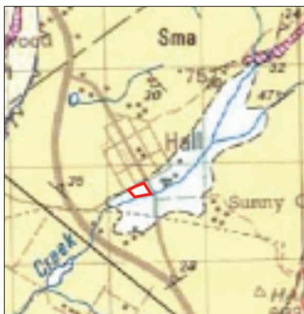
Figure 4. Geology of the Hall Region (image modified from Abell 1993) (Yellow denotes Mount Ainslie Volcanics, white denotes alluvium)
