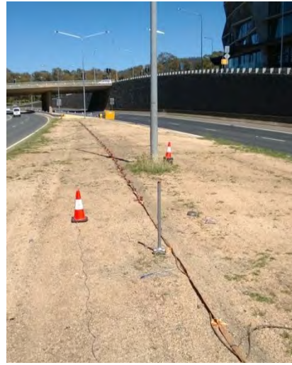
Photo 2 Onsite seismic array with sledgehammer
