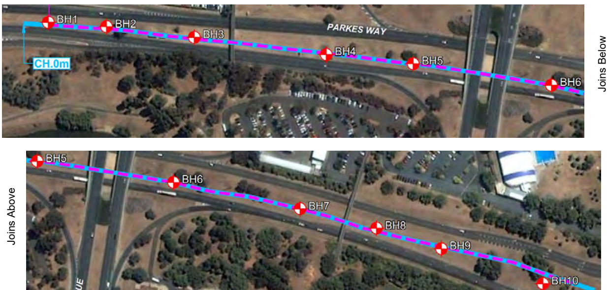
Figure 19 – Parkes Way Borehole Locations
