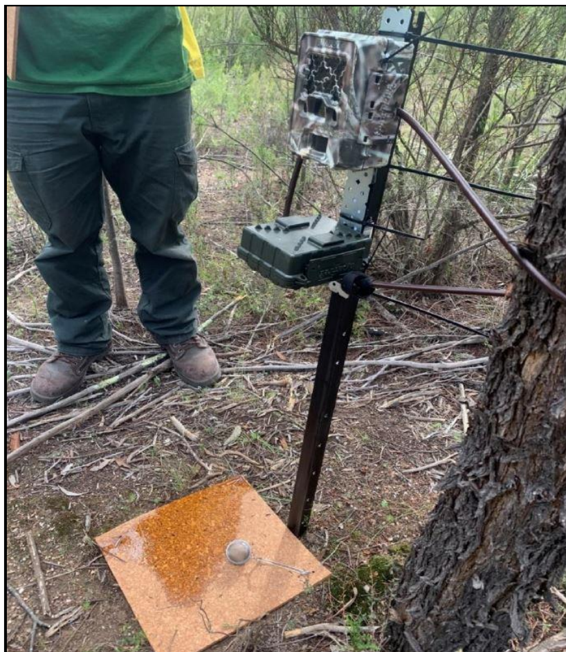
Figure 5. Camera station set up to include a white flash camera (lower), positioned perpendicular to the star picket to capture images of small native mammals, and an infrared camera (upper), positioned vertically to capture images of introduced predators such as cats and foxes. A cork tile is pegged into the ground directly below the white flash camera. In one corner, a metal tea strainer containing an oat and peanut butter bait ball is pegged to the tile to attract native small mammals. A chain lock secures the cameras to the tree.
